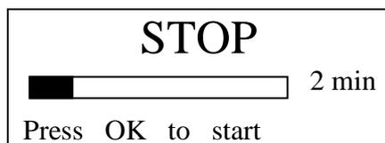
Stop mode is limited to 2 min. After 2 min. an audible alarm is sounded. Press the **STOP/NO** key again, to mute the alarm.
