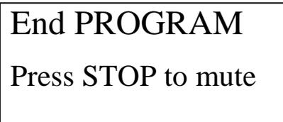
The pump will automatically turn to a **KVO** mode when the program is completed. Press the **STOP/NO** key to reset the pump and set a new program.
