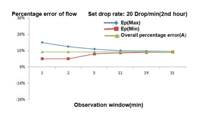
Sampling rate: 20 Drop/ min Sampling interval:  $\triangle$  t =1 min Observation windows:  $p\triangle$  t = 1, 2, 5, 11, 19, 31 mins Maximum deviation over the course of a full observation window: Ep(Max) (%) Minimum deviation over the course of a full observation window: Ep(Min) (%) Average deviation: B(%)
