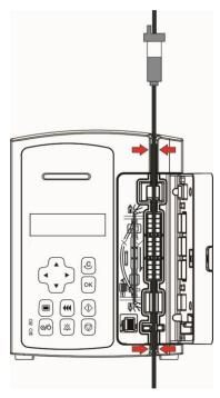
3. Straighten the infusion set, align the central tube seat, put it in flatly, and install the infusion set as shown in the figure.
