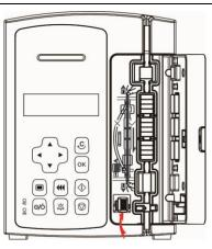
2. Pull the liquid check clip button upward left, and open the liquid check clip.
