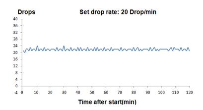
Sampling rate: 20 Drop/ min Sampling interval:  $\triangle$  t =1 min Observation windows:  $p\triangle$  t =1, 2, 5, 11, 19, 31 mins Maximum deviation over the course of a full observation window: Ep(Max) (%) Minimum deviation over the course of a full observation window: Ep(Min) (%) Average deviation: A (%)
