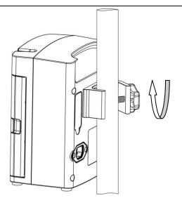
2. Tighten the pole clamp clockwise to firmly fix the device on the IV stand (round vertical bar with diameter size of 15-32mm).
