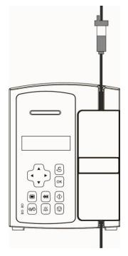
4. Close the door, the interface will enter [Infusion set selection] interface, indicating that the infusion set is installed correctly; otherwise, it needs to be reinstalled.
