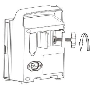
1. Turn counterclockwise to loosen the pole clamp until an IV stand can be inserted in.
