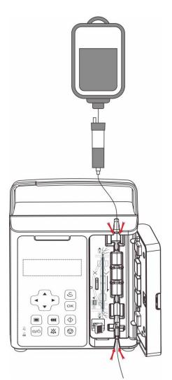
3. Load the set, confirm it is firmly loaded into the 4. Close the door, the interface will enter tube slot. [Infusion set selection] interface, indicating
