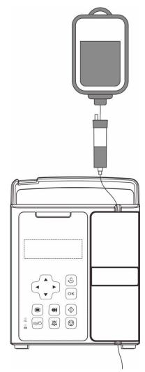
4. Close the door, the interface will enter **[Infusion set selection]** interface, indicating that the infusion set is loaded correctly; otherwise, it needs to be reloaded.
