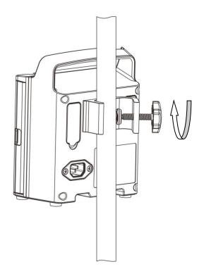
2. Tighten the pole clamp clockwise to firmly fix the device on the IV stand (round vertical bar with diameter size of 15-32mm).
