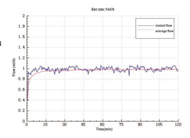
Syringe brand: Dove Syringe specification: 20ml Sampling quantity of pump: 3 Sampling quantity of syringe: 3
