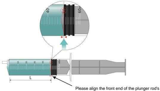
Please align the front end of the plunger rod's sealing plug with the full dimension mark
